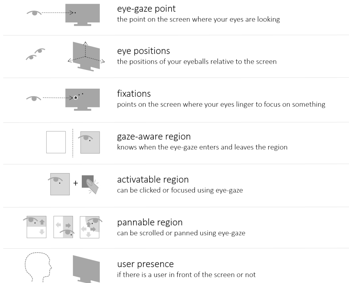
Figure 1 A somewhat simplified view of what the EyeX Engine API can do for you.
